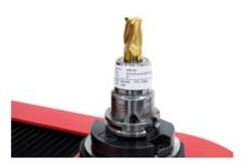
**Label Printing:** You will receive five measurement results precisely and reliably in seconds, with length, diameter, radius, and angle 1 and 2 for the tool cutting edge.
