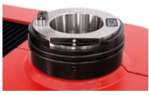
**SK50 Tool Holder Spindle** with high concentricity and integrated calibration edge.
