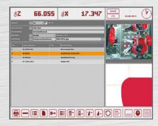
Data output in a format appropriate for the tooling machine controller (DOP), including format generator to generate post-processors / output formats (over 100 output formats are included in the EZset DOP library)
