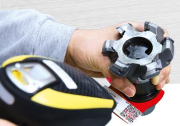
With the EZset identification code »zidCode«, you save up to 45% more time in comparison to manually entering actual tool data into the machine controller. Input errors are also avoided entirely – time-consuming reworking is eliminated, and process security is increased.
