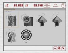
Standard programs for specialized measurement tasks with clear presentation of tool parameters and input fields
