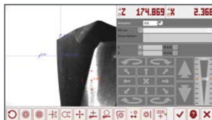
Tool cutting edges in incident light with 40x zoom to inspect cutting edges for wear and tool breakage
