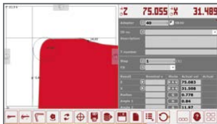
User-independent measurements with dynamic cross hairs and automatic cutting edge shape recognition
