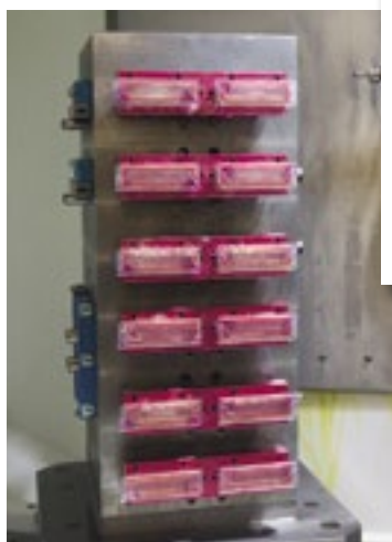
DoveLock jaws used for glass machining
