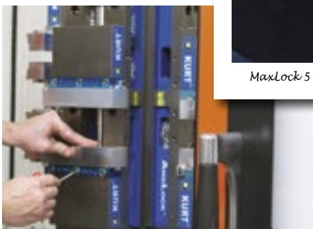
DoveLock jaws provide 1 minute changeover
