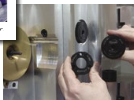
PinLock locating system installed in a tombstone
