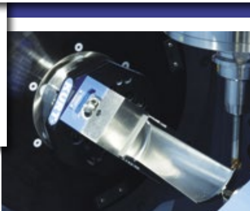
MaxLock 5 axis vise used for turbine blade machining
